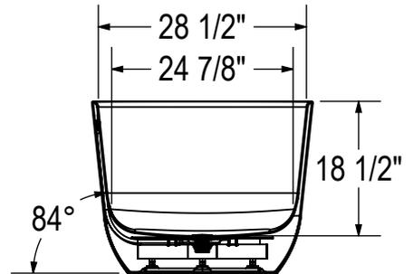
All dimensions are approximate. Structure measurements must be verified against the unit to ensure proper fit.
