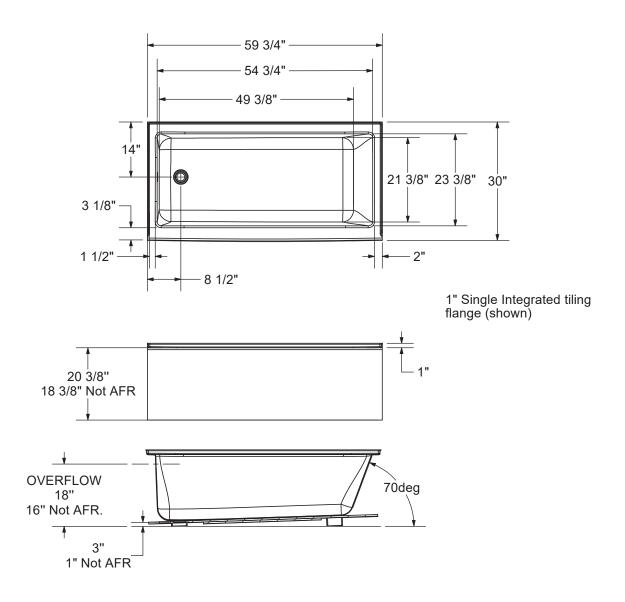
Wood support design may vary. Single Integrated tiling flange: 1" height x 1/4" thickness (shown)
