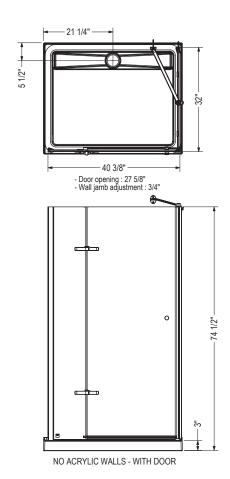
**Dimensions:** - x 78 3/4 in. (- x 2000 mm) **Glass Thickness:** 1/4 in. (6 mm) Weight: 180 lbs (81.63 kg) Minimum access: (mm) Maximum access: ( mm)
